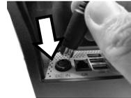
4. Have the cover join to the wedge portions of the bottom I/O interface.
