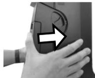
9. After ensuring the front cover is well attached to the rear case, insert the two screws back into the screw holes inside the compartment, secure them, and then close the cover.
