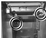
10. Insert the screw which you removed in step 1 to the screw hole at the bottom, and then fasten it properly, as the figure shows.
