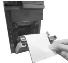
6. Make sure the paper roll is well loaded with the end of the paper sticking out as shown in the figure.
