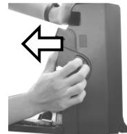
5. From the left-hand side of the terminal, remove the front cove from the rear case.
