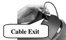
6. Press down the cover to close the bottom I/O interface chamber.
