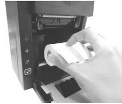
4. Unroll the thermal paper and drag the loose end of the paper till it extends towards the paper cutter.
