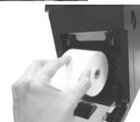
3. To load the thermal printer with **the 3-inch paper roll**, just drop the thermal paper roll inside the paper roll compartment of the printer as illustrated in the figure.
