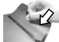
5. Before pushing the cover back into place, neatly thread the cables through the cable exit.
